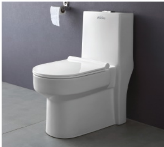
LAVISH L-645, W-360, H-745mm | 'S' Trap -Distance -9.00" 'P' Trap -Distance -7.20" Flushing -Washdown ₹ 14000/-
